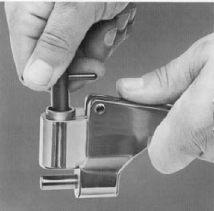
FIG. 3 Adjusting load on load spring
